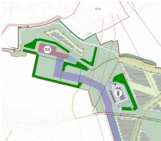
Figure 15.7 -- Onsite Substation and BESS Compound Extract from Figure 2.1 - Indicative Site Layout [EN010163/APP/6.4.1]
